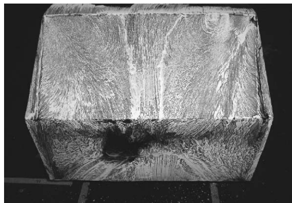
Fig. 13. Rear end surface skin friction patterns.
